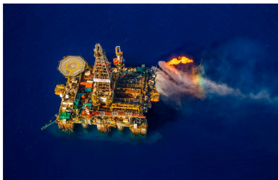
Drill stem testing at the Aphrodite field in Cyprus' exclusive economic zone.
